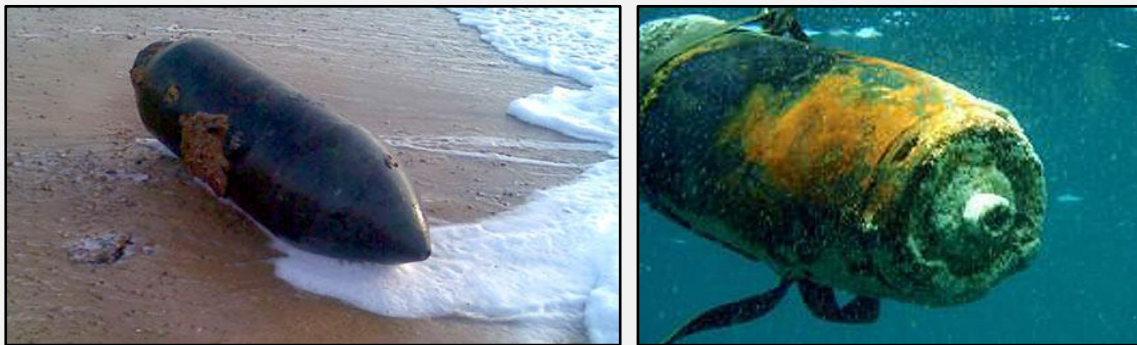
German (R) and British (L) HE bombs as UXO (note typical absence of tail)
